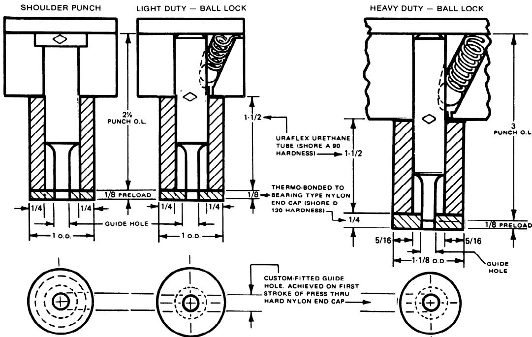
For special thickness retainers or special length punches, the Uraflex® portion of the Nomar™ Stripper can be machined to a shorter length to provide for preload or can be ordered to custom length.
